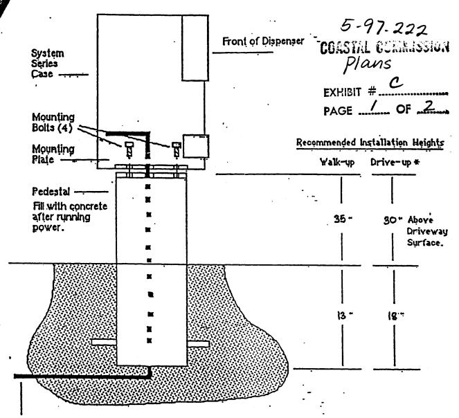
115 Volt/15 Amp (min) service. It is recommended that consideration be given to a twisted pair of 18 ga. wires for an exterior alarm, future communications and/or gate signal wires. Any of these should be shielded and in separate conduit.
