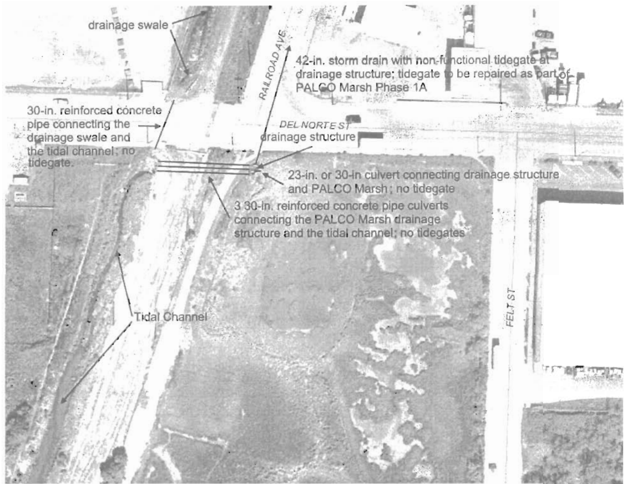
Figure 1. Overview of northwest outlet from Palco Marsh to the Tidal Channel. Note the former Eureka Plywood Mill drains to the drainage swale in the upper left of the photo. The bay is at the south end of the Tidal Channel, about 800 feet beyond the lower left corner of the photo.
