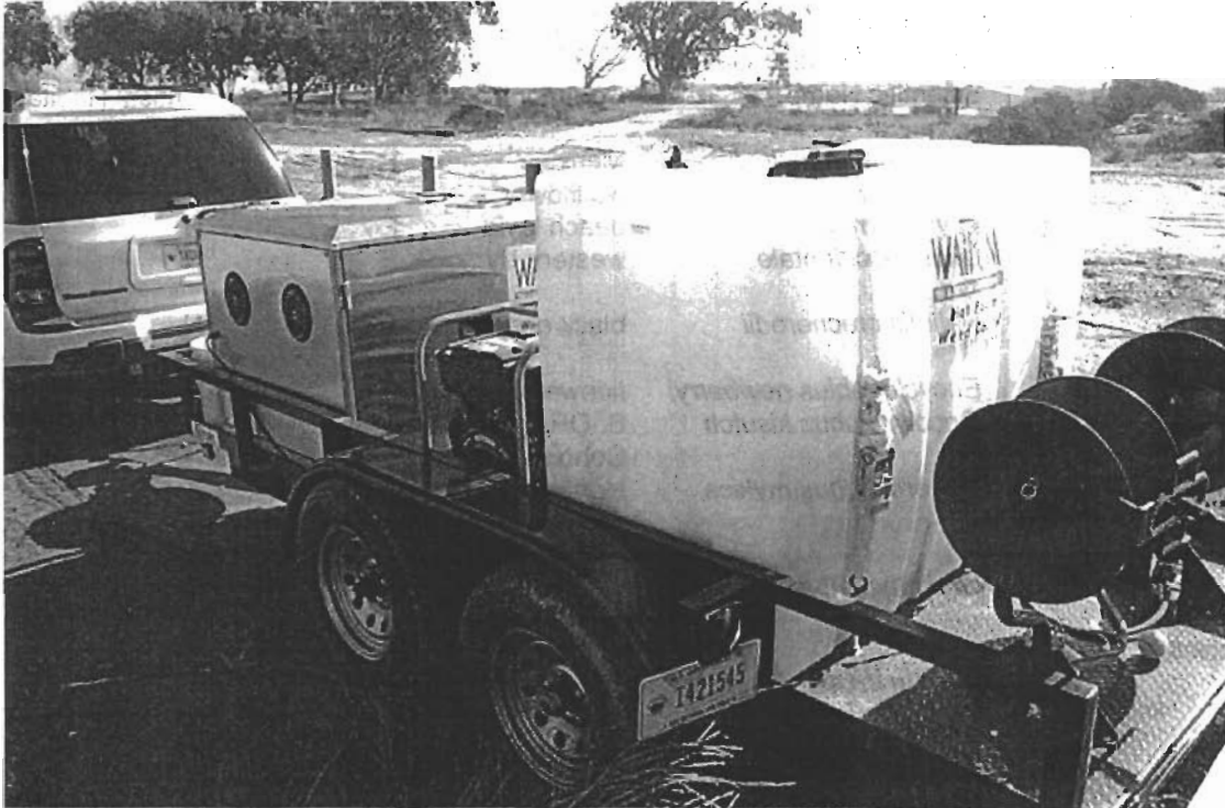
Figure 9. The Bureau of Land Management's hot water weed control system, called the Waipuna.
