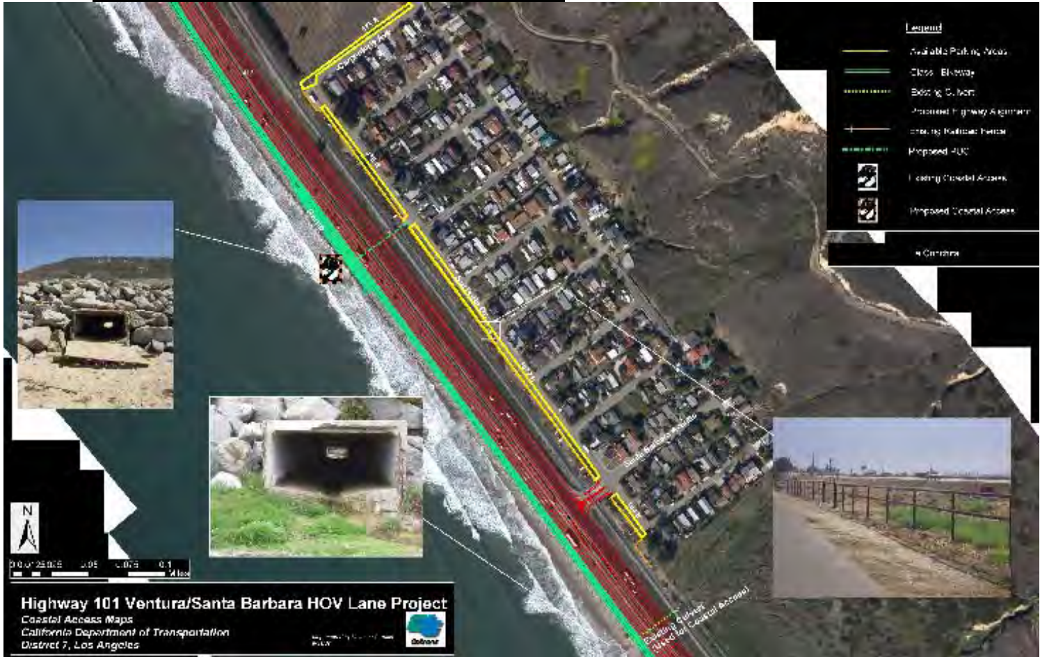
Existing box culverts, proposed Coastal Trail/bikeway, new pedestrian undercrossing (PUC) location, & perimeter parking at La Conchita
