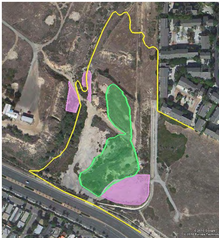
Figure 1. The yellow line represents the proposed limits of grading for the Sunset Ridge entrance road and parking lot; grading for the rest of the park would extend off to the southeast. Green screen shows an "island" of coastal scrub and grassland that would be preserved under the proposed grading plan. Pink screen shows three areas cleared in 2004 without a coastal development permit. Proposed grading overlaps entirely with the Southeastern Polygon, partially with the Northeastern Polygon, and is adjacent to the Northwestern Polygon.
