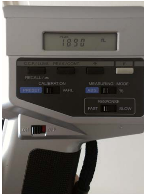
Photo 2: Minolta LS-100 Luminance Meter, Display Setting for Output foot lamberts (fL)
