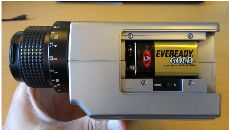
Photo 3: Minolta LS-100 Luminance Meter, Switch Set for foot lamberts (fL).
