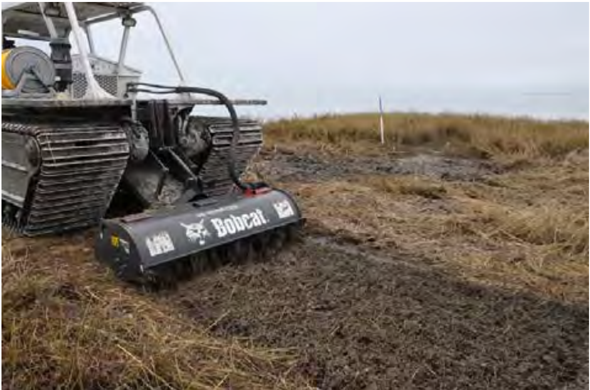
Photo 2. Marsh Master with rototiller attachment following a top mow on the Humboldt Bay National Wildlife Refuge. Photo courtesy of the HBNWR.
