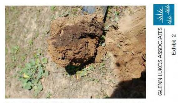
Photograph 5: 2.5 inch thick layer of Asphaltic material in C Extended 3.
