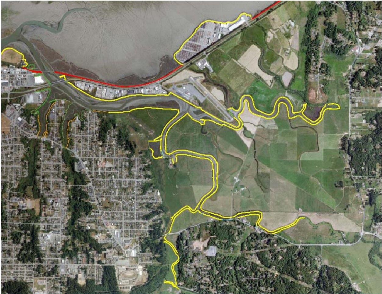
Figure 8. Shoreline structure on Eureka Slough is predominately made of dikes (yellow) built in the 1890s to convert former tidelands to agricultural uses.
