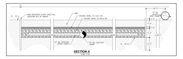
Figure 3.6 Section of SIG using float-in construction methods
