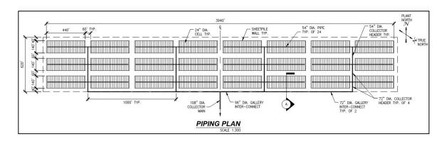
Figure 3.5 Plan of SIG using float-in construction methods
