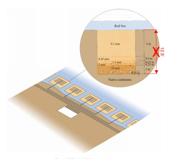
Figure 3.2 Typical SIG cross-section
