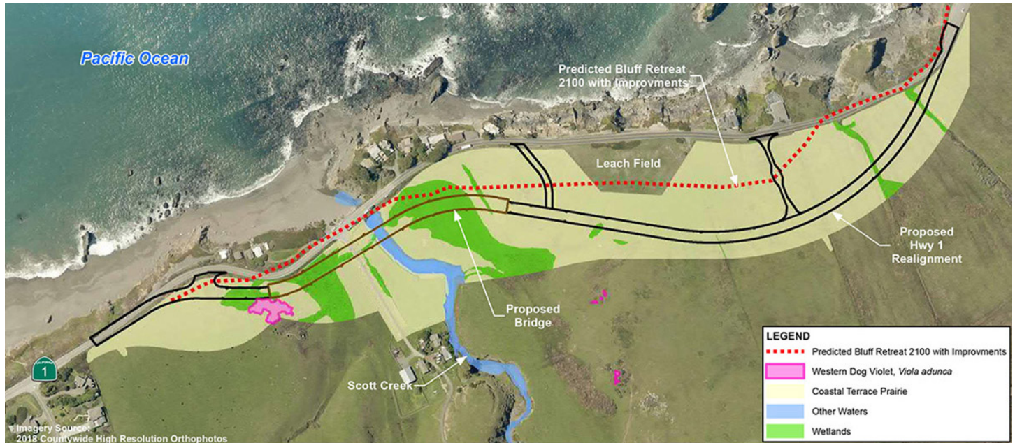
Image 10. Realignment diagram of Highway 1 near Gleason Beach in Sonoma County. Photo by Caltrans .
