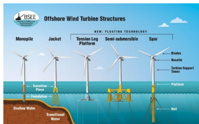
Diagram of offshore wind turbine structures. Current wind energy areas would utilize floating technology - either tension leg platform, semi-submersible, or spar. Source: Bureau of Safety and Environmental Enforcement
