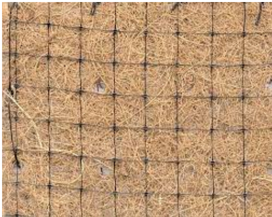
Coir erosion control blanket with plastic netting
