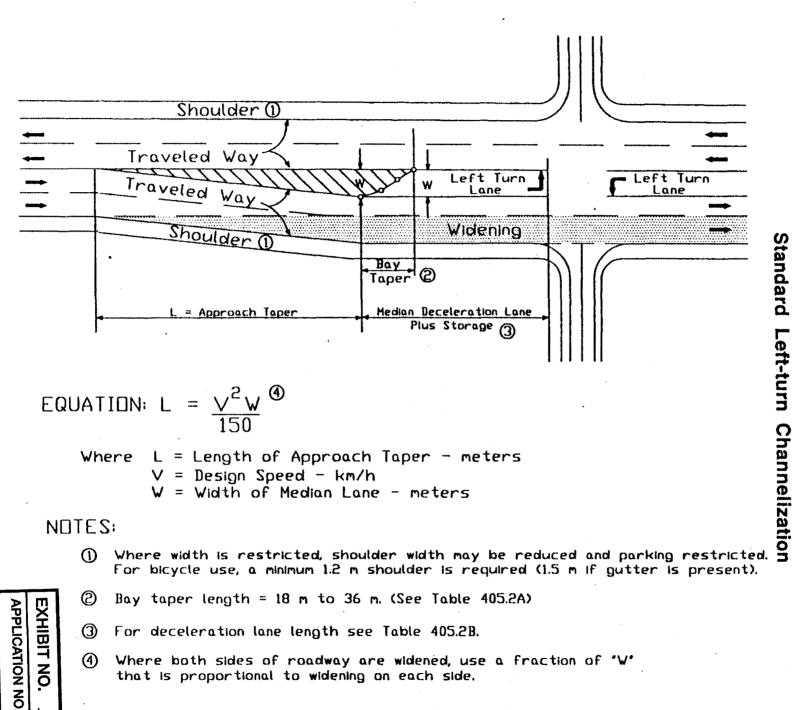
(4) Where both sides of roadway are widened, use a fraction of "V" that is proportional to widening on each side.
