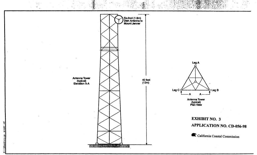
The proposed six-foot (1.8m) dish antenna would be near the summit of the new 40-foot (12m) tower. This antenna would be oriented north-northwest towards Mount Jenner.
