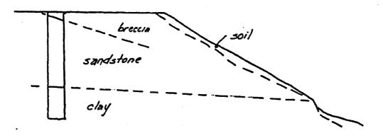
The above section oriented N20W indicates an apparent dip of about 3 degrees in the downslope direction. Exposures on the adjacent property indicate this is roughly also the true dip.
