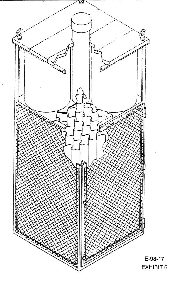
This cut-away drawing shows the cages design used for the larger abalone (2 - 3.5). These are 4' x 4' x 10' tall and can hold up to 5,000 animals. The tube at the top is for adding kelp.
