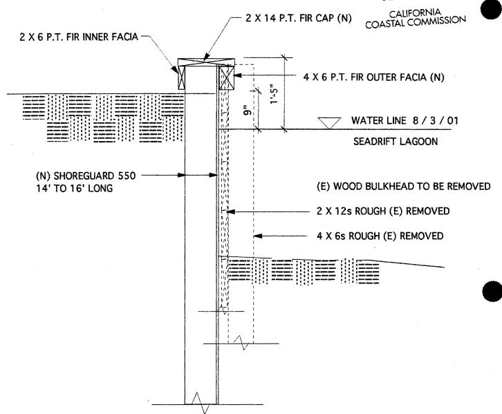
SECTION THROUGH (N) BULKHEAD (VINYL SHEET PILES)
