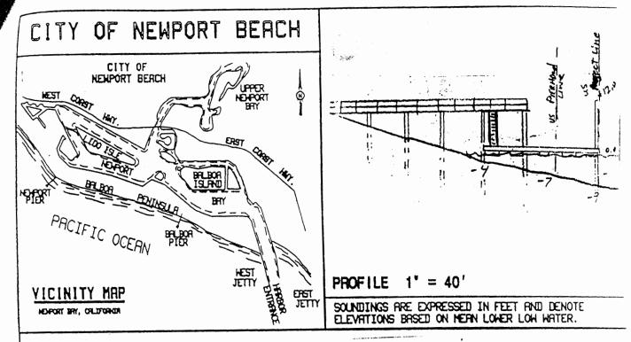
Scope of work: Remove west finger of existing float. Install new 8' x 49' finger and 4'x 22' back walk so that slip is 22' wider than existing configuration. Install one new 16" pile and relocate one 14" pile. Existing approach, pier and gangway remain with no configuration change.
