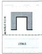
C. Open Courtyard: an Open Courtyard is a court that is surrounded on three sides by a "U"-shaped building. The fourth side is completely open to the street.
