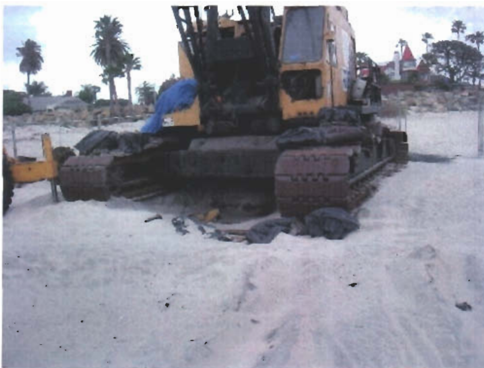
Trash by cranes, no barrier for dripping fluids (and dropping solids)
