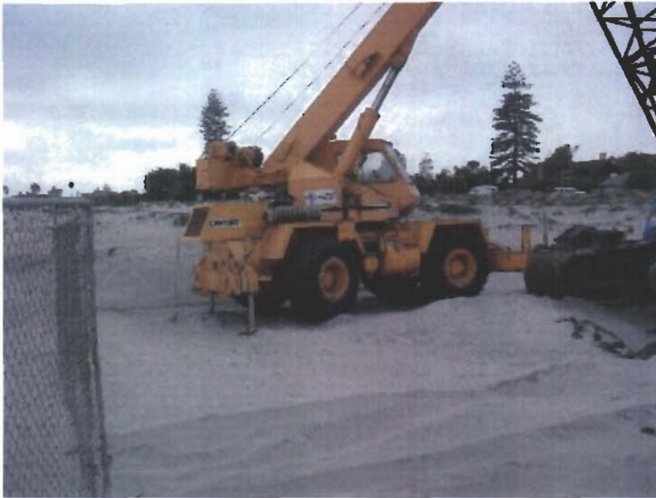
No barrier under the smaller crane, hydraulic levelers directly on the sand.
