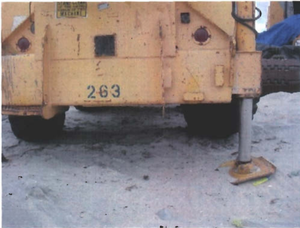
Detail of no barrier under smaller crane with debris scattered under and around it
