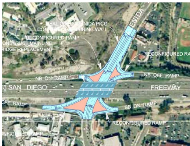
Figure 12: Single Point Diamond Interchange Concept at I-5/Avenida Pico Interchange
