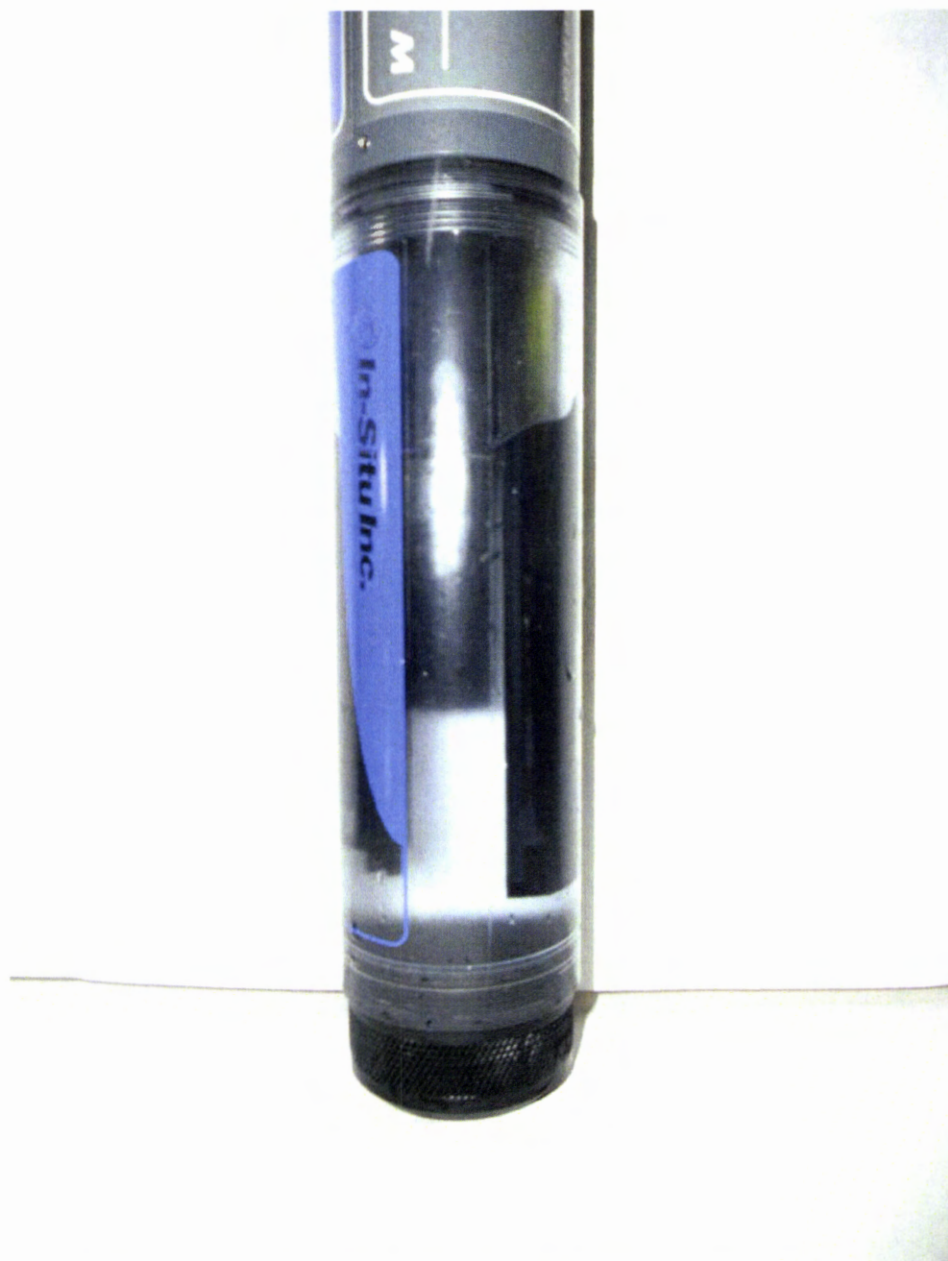
Photo 2: Turbidity of 14.4 FNU that is not noticeable within instrument when held at arms length.
