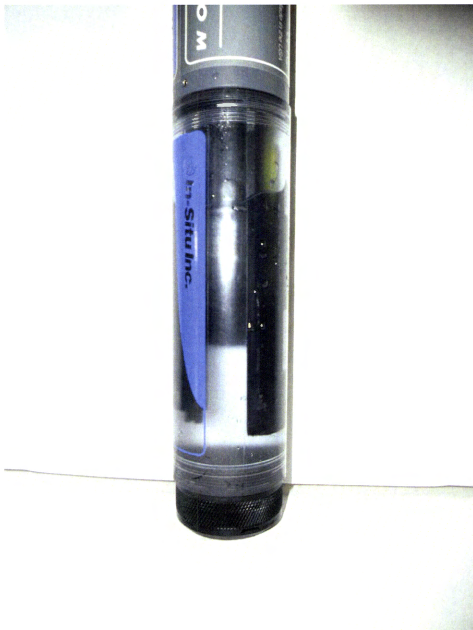
Photo 1: Turbidity of 9.1 FNU that is not noticeable within instrument when held at arms length.
