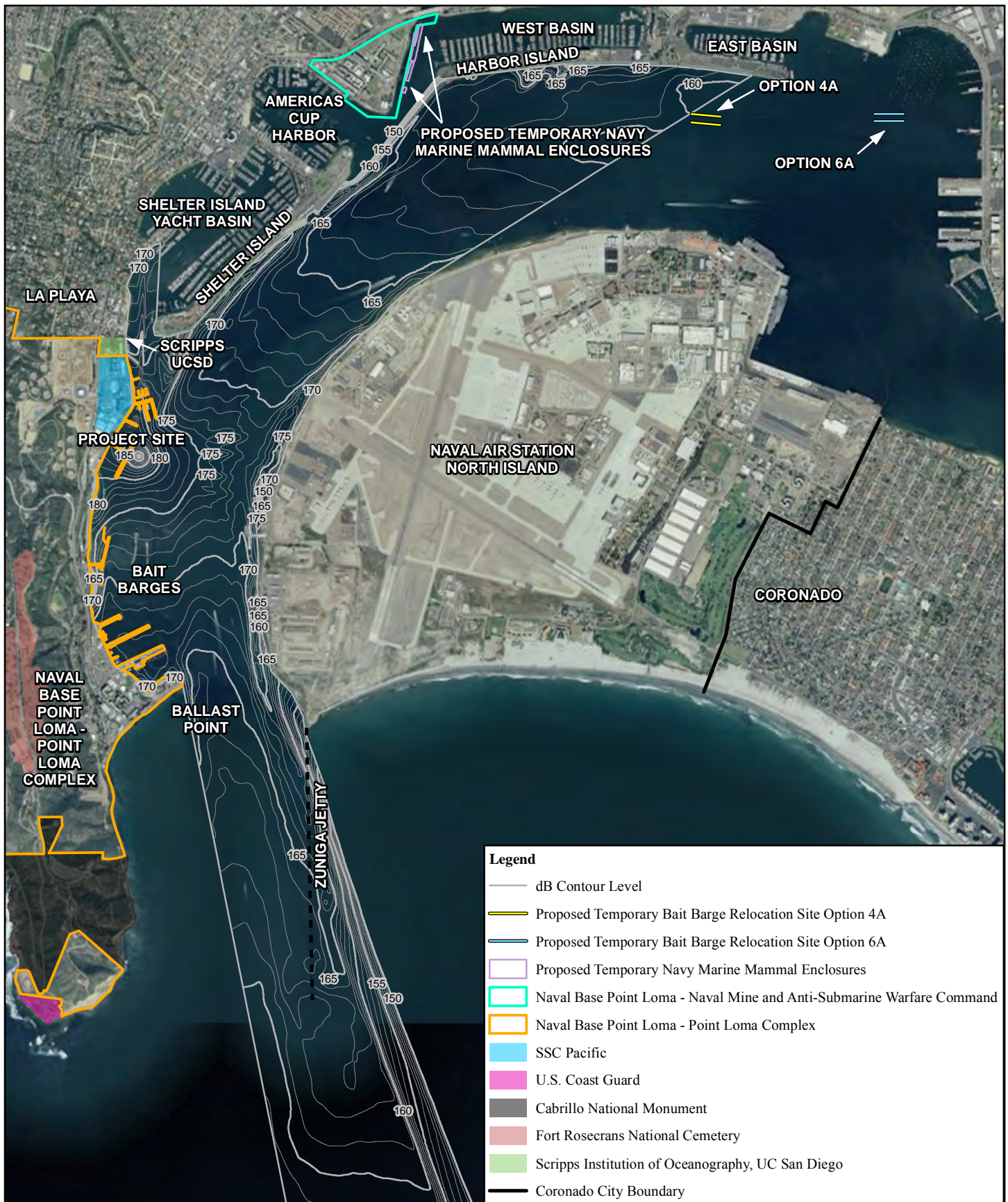
Figure 3.2-1 Underwater Sound from Impact Pile Driving, 36-48 " Steel Piles (Source = 195 dB rms)
