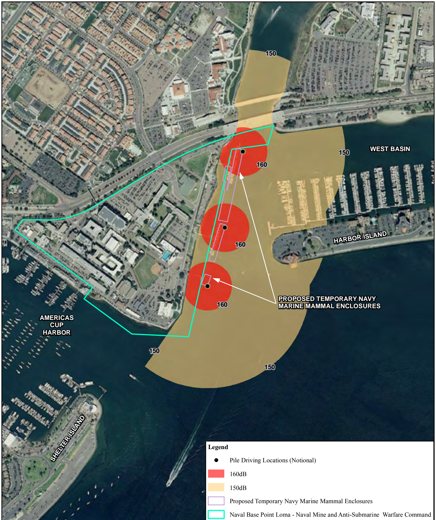
Figure 3.2-5 Underwater Sound from Impact Pile Driving at Marine Mammal Relocation Site, 18" Concrete Piles (Source = 173 dB rms)
