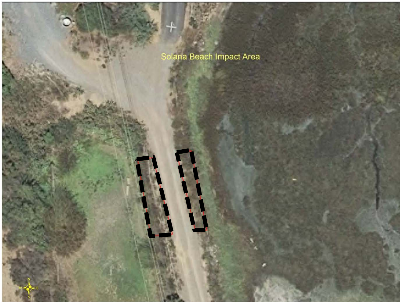
Figure 2. Impact area along the roadside calculated at 40' \times 5' and 40' \times 6' = 440 sq. ft. At a ratio of 3:1, the restoration area should = ~0.03 acres (1,320 sq. ft.)
