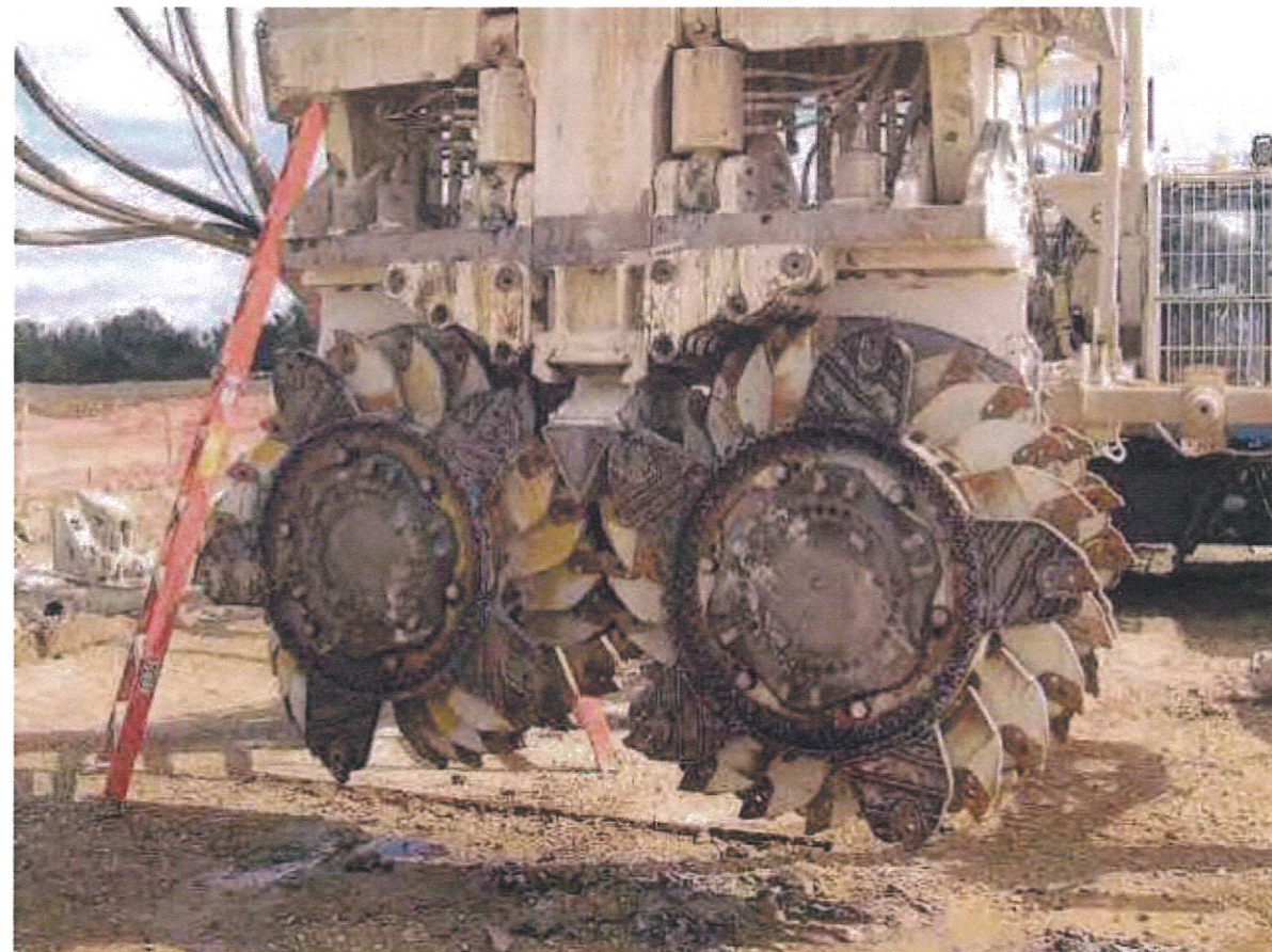
Hydromill Cutting Head
