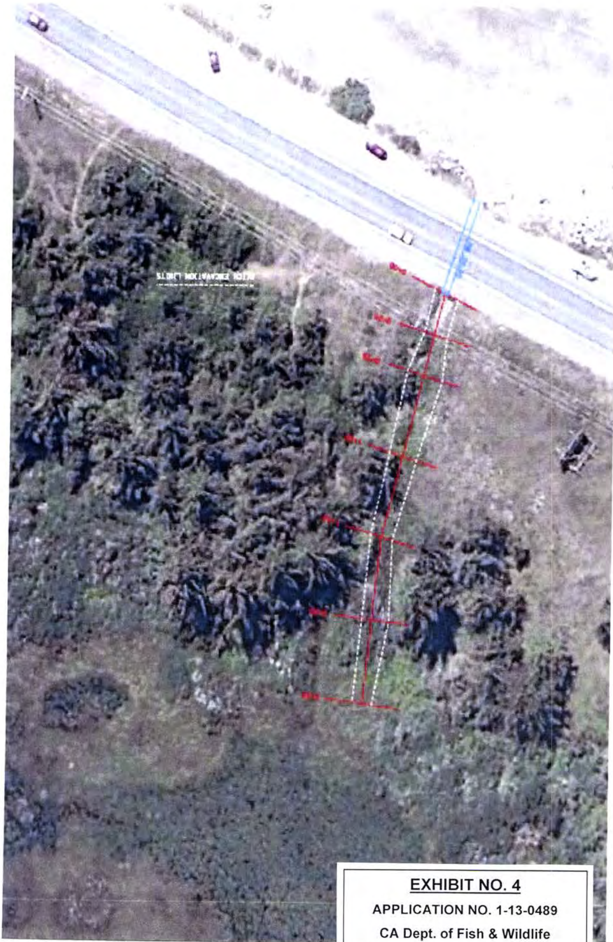
Figure 9. Aerial view of the North Ditch that matches the cross-section design found in Caltrans Figure 4A, Figure 4B, and Figure 4C of previous documents. This is the corridor that the excavator will follow as it cleans out the ditch and side-casts the material along both sides of the ditch. There will be no impact to sedge marsh vegetation (see text, Figure 1 and Figure 2). Dashed line are the ditch excavation limits.
