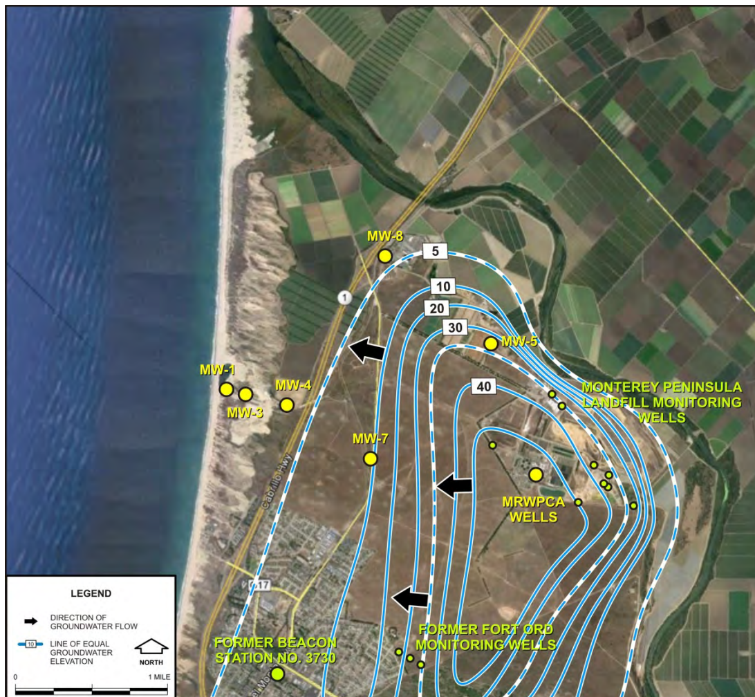
Figure 7 – Dune Sand Aquifer Groundwater Elevation Contour Map
