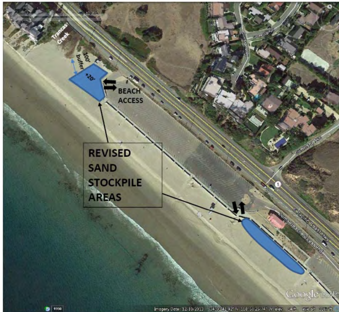
Figure 15. Construction Staging & Stockpile Areas For Alternative 4C Project
