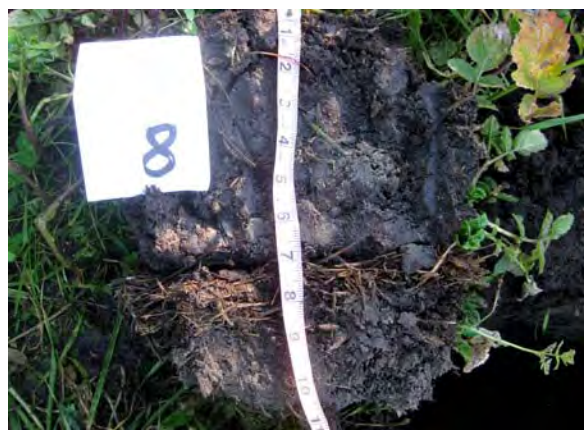
Photograph 4. Fill profile at Pit #8 showing 7 inches of loamy fill soil on top of decomposing surface vegetation, underlain by original sand.
