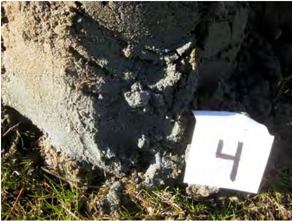
Photograph 1. Soil Pit #4 revealing nearly pure sand with stray pieces of scrap metal simulating redoximorphic features. Notice small piece of iron in upper left corner.
