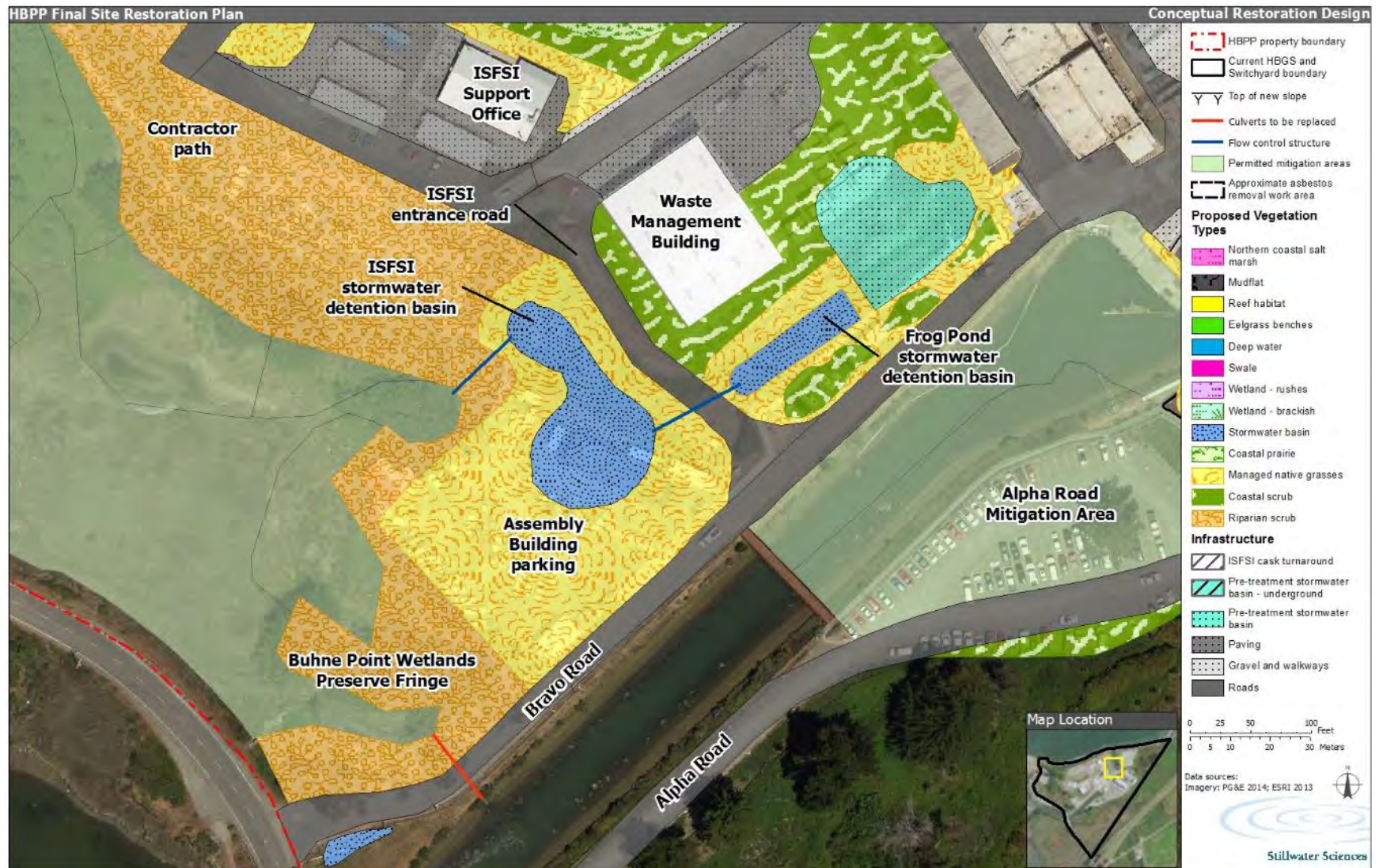
Figure 7. Proposed conceptual design for the Assembly Building and ISFSI and Frog Pond stormwater detention basins.
