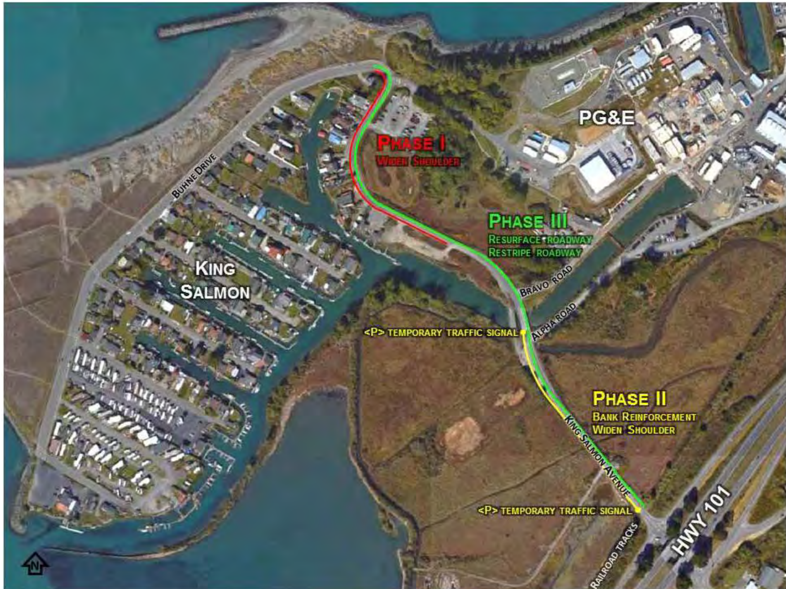
Figure 1-4. King Salmon Avenue shoulder widening project area and work phases.
