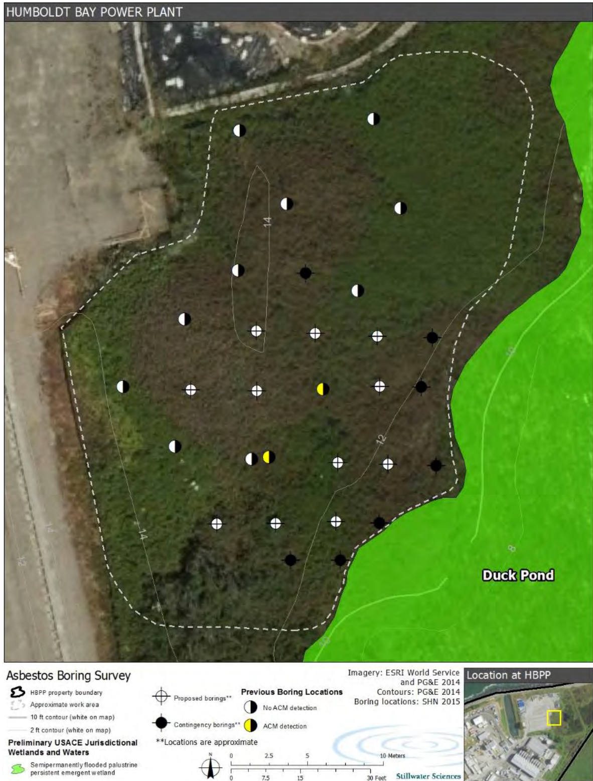
Figure 3. Asbestos-containing material (ACM) removal work area.
