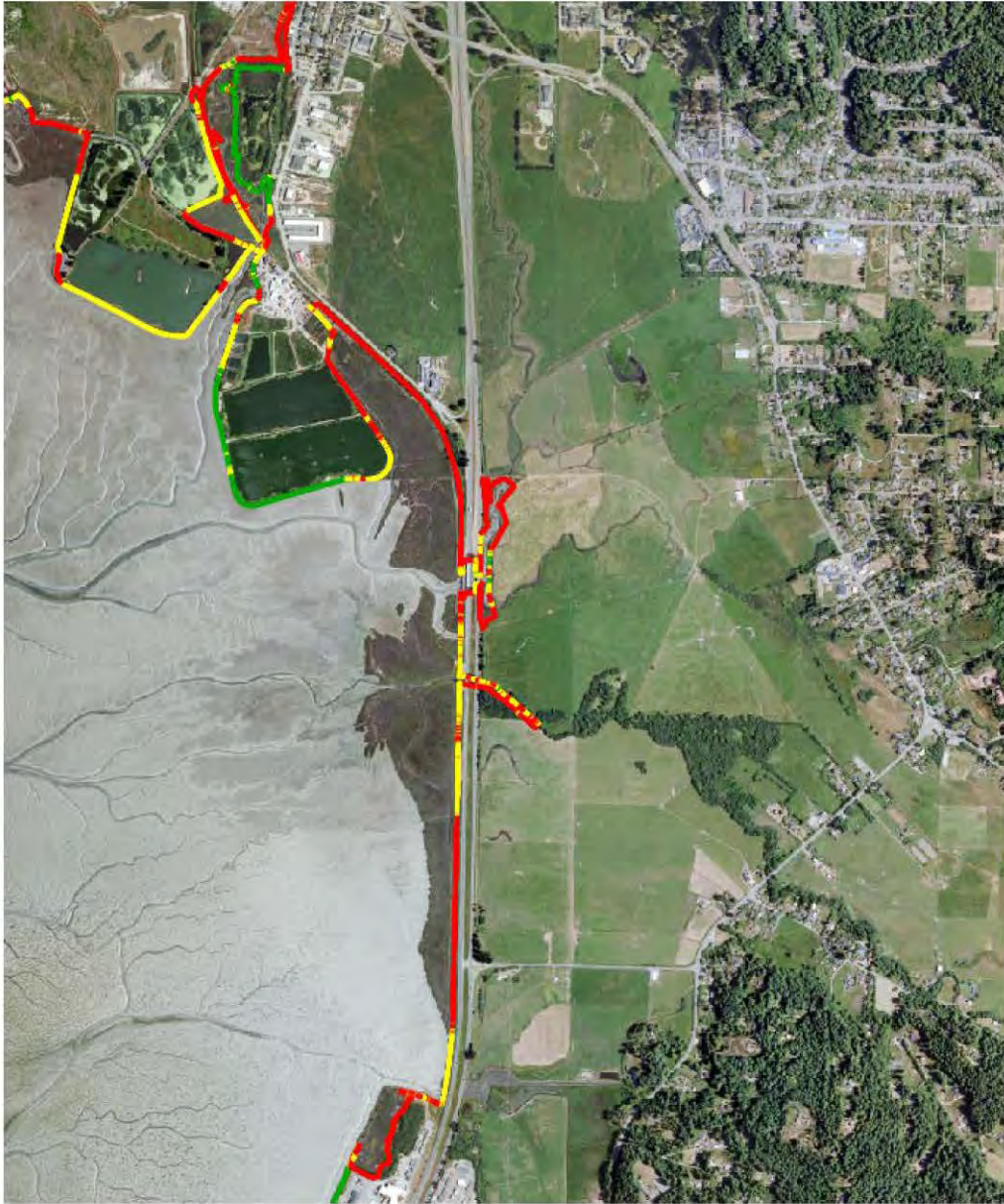
Figure 10. Shoreline vulnerability rating of the upper reach of Highway 101: high (red), moderate (yellow), and low (green) (Powell 2013).
