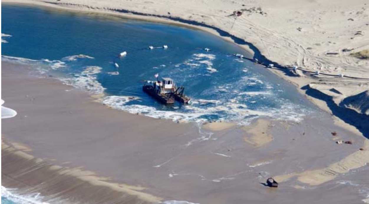
Figure 3. Image of the sand mining operations at the CEMEX Lapis Mine. Note the fact that waves are pouring over the berm and into the lagoon. Effectively, the mining here is occurring in the active surf zone. Photo credit: Gary Griggs
