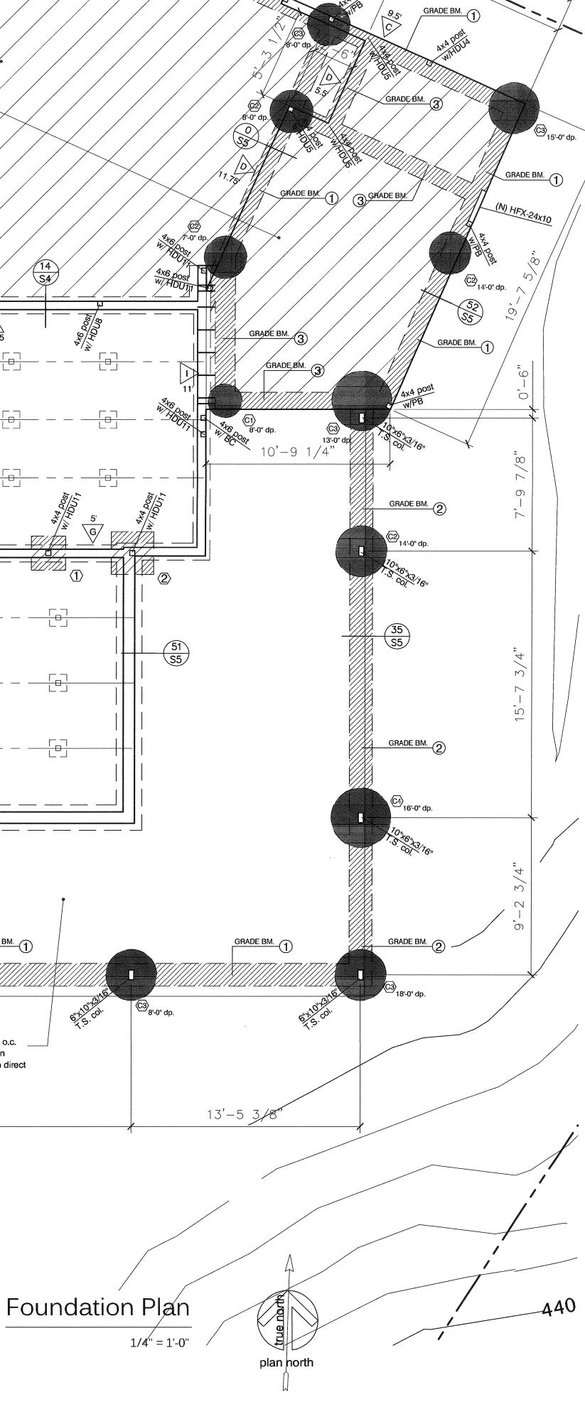
A. All footings shall be founded into natural undistrubed soil as per Code (2010 C.B.C. Table 1804.2. Bearing value is assumed to be 1500 psf).
