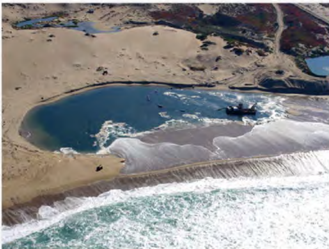
Dredge pulls sand from the CEMEX Sand Mine in Marina
