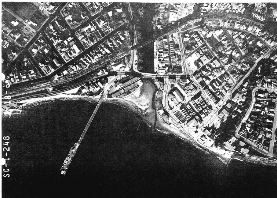
Figure 2: Aerial of Capitola Beach in 1967 after construction of Jetties at Santa Cruz and Prior to Construction of Capitola Jetty (source: USACE 1971)
