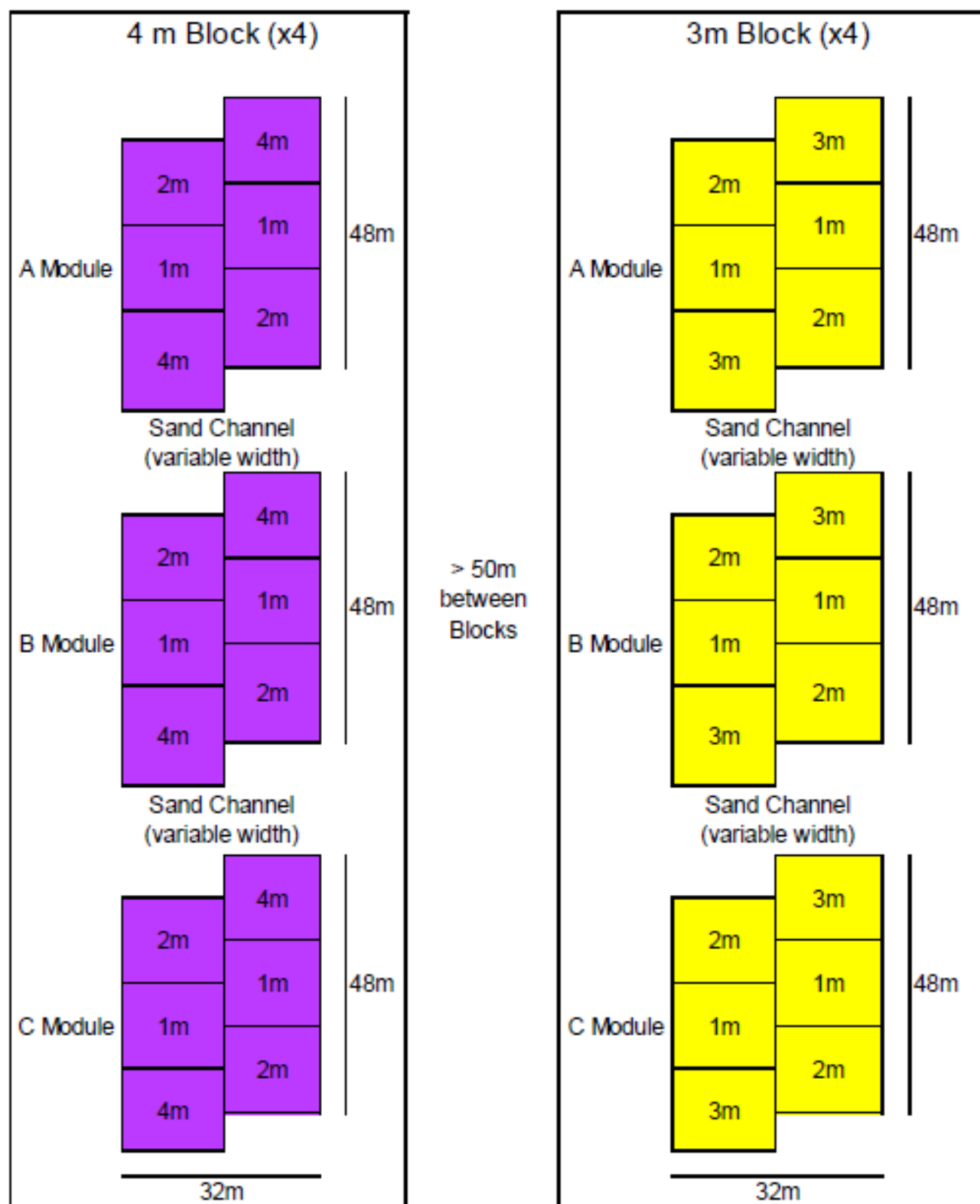
Figure 23. Design of 3m blocks and 4m blocks. Each block contains three modules (A, B, C). Each module consists of a 3 x 2 set of piles, offset by 1/2 pile length. Each pile is a 16 m x 16 m square pyramid of quarry rock with the overall height listed. There is a 10 to 20 m wide sand channel between modules and at least 50 m of space between blocks (construction design, control and precision details are contained in Appendix D).
