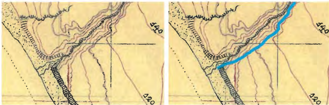
Figure 2. Detail of Trafalgar Canyon, with southern canyon edge added in blue to show the approximate transition between the coastal terrace gently sloping toward the ocean and the canyon edge where the slope is northwest and steeper down into the canyon.
