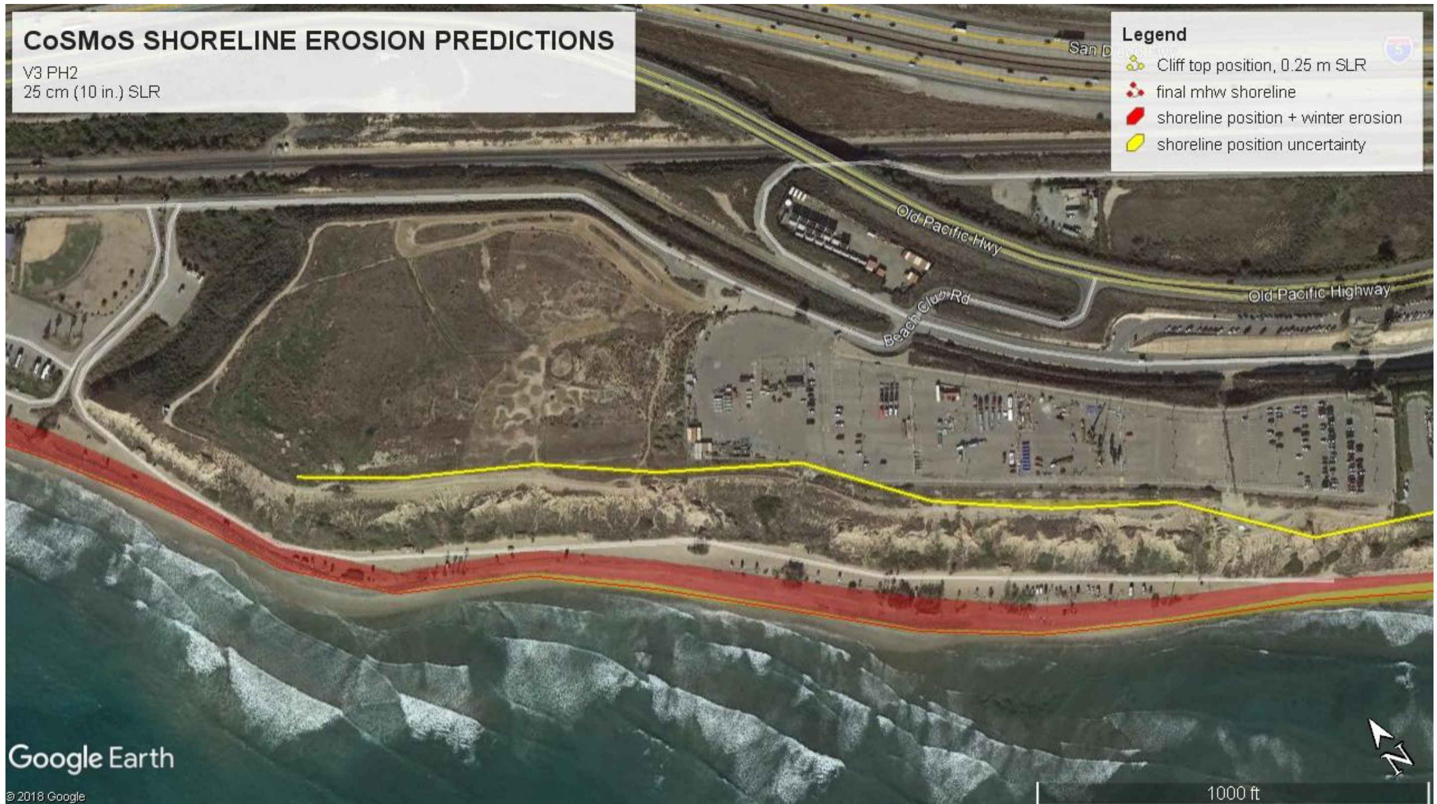
FIGURE 5.4: CoSMoS SHORELINE EROSION PREDICTIONS – 0.8 FT (10 IN. / 25 CM) SLR
