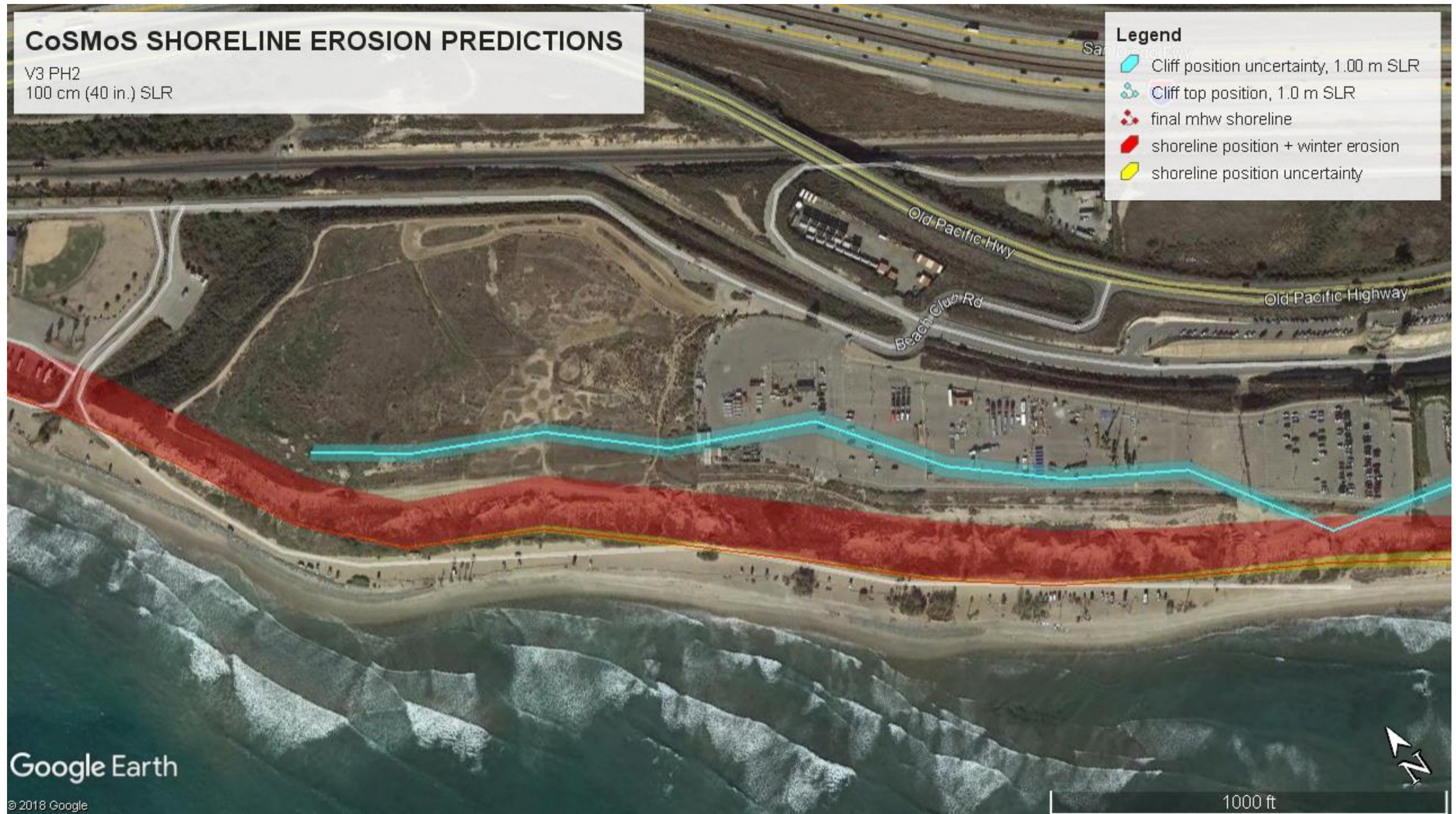
FIGURE 5.6: CoSMoS SHORELINE EROSION PREDICTIONS – 3.3 FT (40 IN. / 100 CM) SLR
