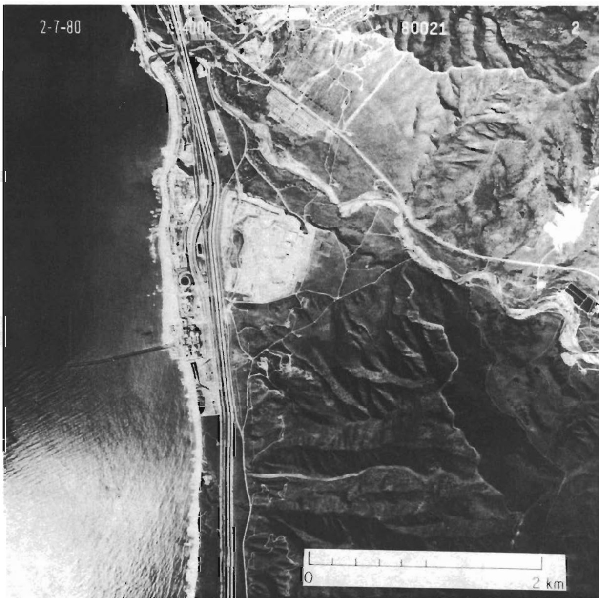
Figure 22. Aerial photograph of reach from San Onofre Creek to south of SONGS taken 7 February 1980. Note beach in front of laydown pad suggesting active sand bypassing at this time which limited upcoast beach width as well as downcoast erosion.
