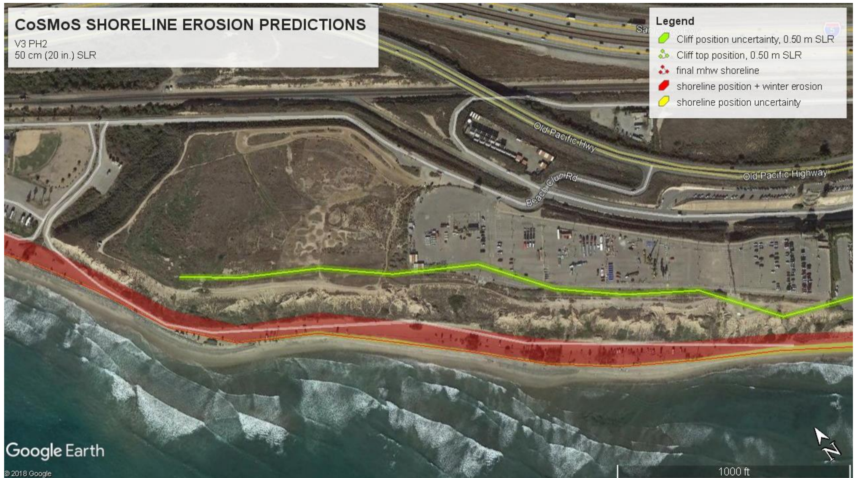
FIGURE 5.5: CoSMoS SHORELINE EROSION PREDICTIONS – 1.6 FT (20 IN. / 50 CM) SLR
