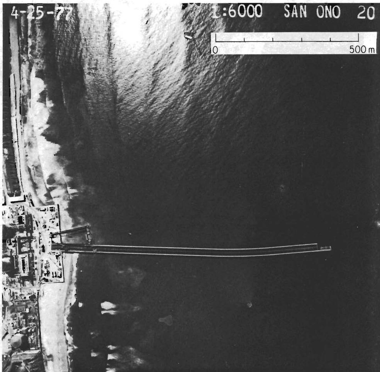
Figure 21. Aerial photograph of beach trestles used to lay Units 2 and 3 cooling pipes. Photo taken 25 April 1977. Note widened fillet beach upcoast of (below) laydown pad beginning to bypass the structure.
