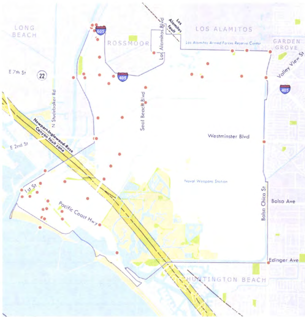
Figure 3-9: Fault Rupture Potential (Newport-Inglewood Fault)
