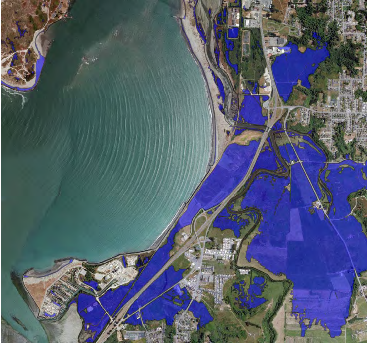
Figure 29. Middle segment with 0.9 ft. of sea level rise with a tidal elevation of 8.8 feet (MAMW). The protective shoreline structures to the east have been compromised. The land adjacent to the road prism is inundated from east of Highway 101, but no lanes become tidally inundated.
