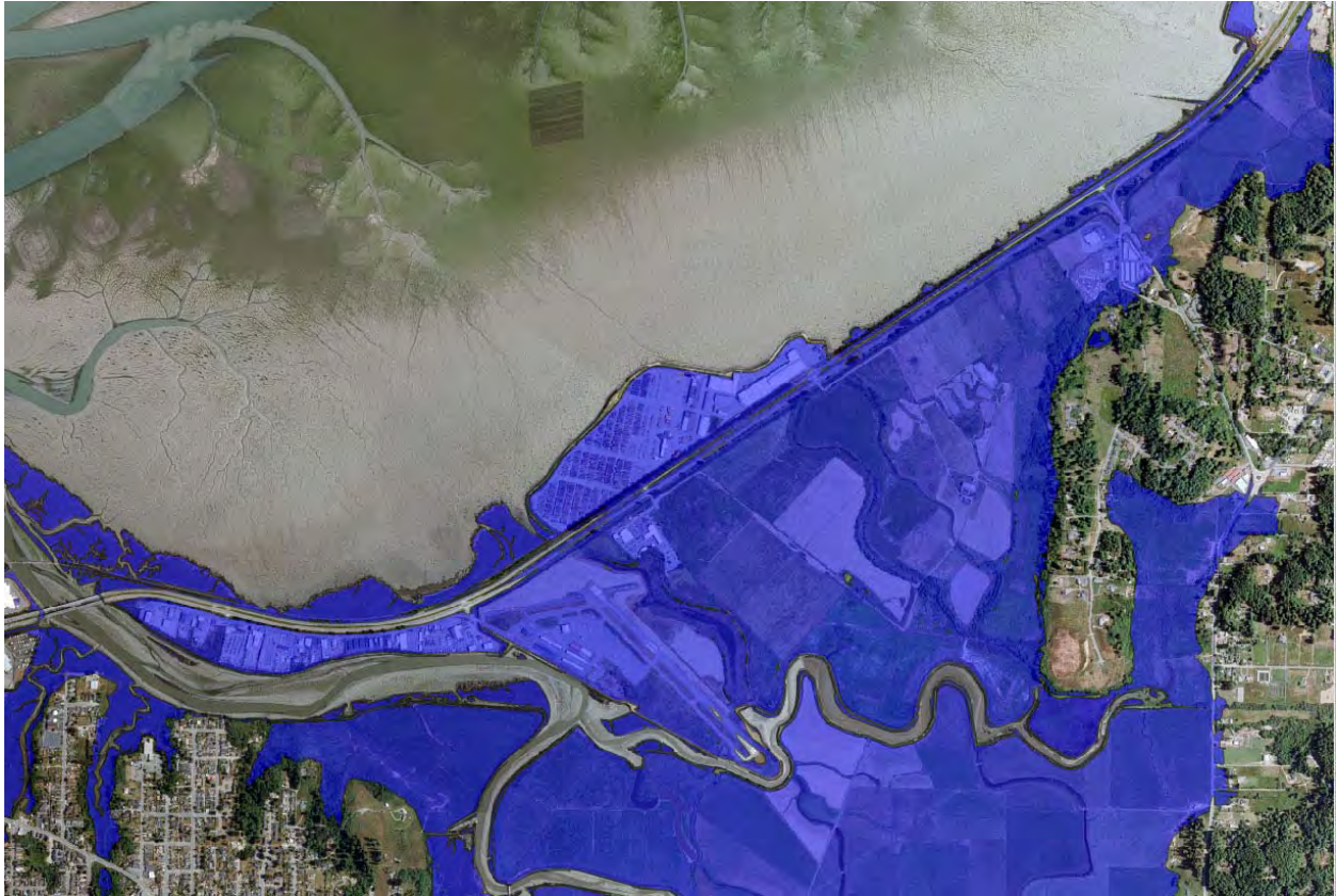
Figure 31. Lower reach of the Arcata Bay segment with 1.6 ft. (0.5 M) of sea level rise and a tidal elevation of 9.3 feet. Protective shoreline structures are overtopped on both sides of the highway, and the road prism is inundated. Approximately 2.0 miles of the north and south bound lanes of the lower reach could become tidally inundated.
