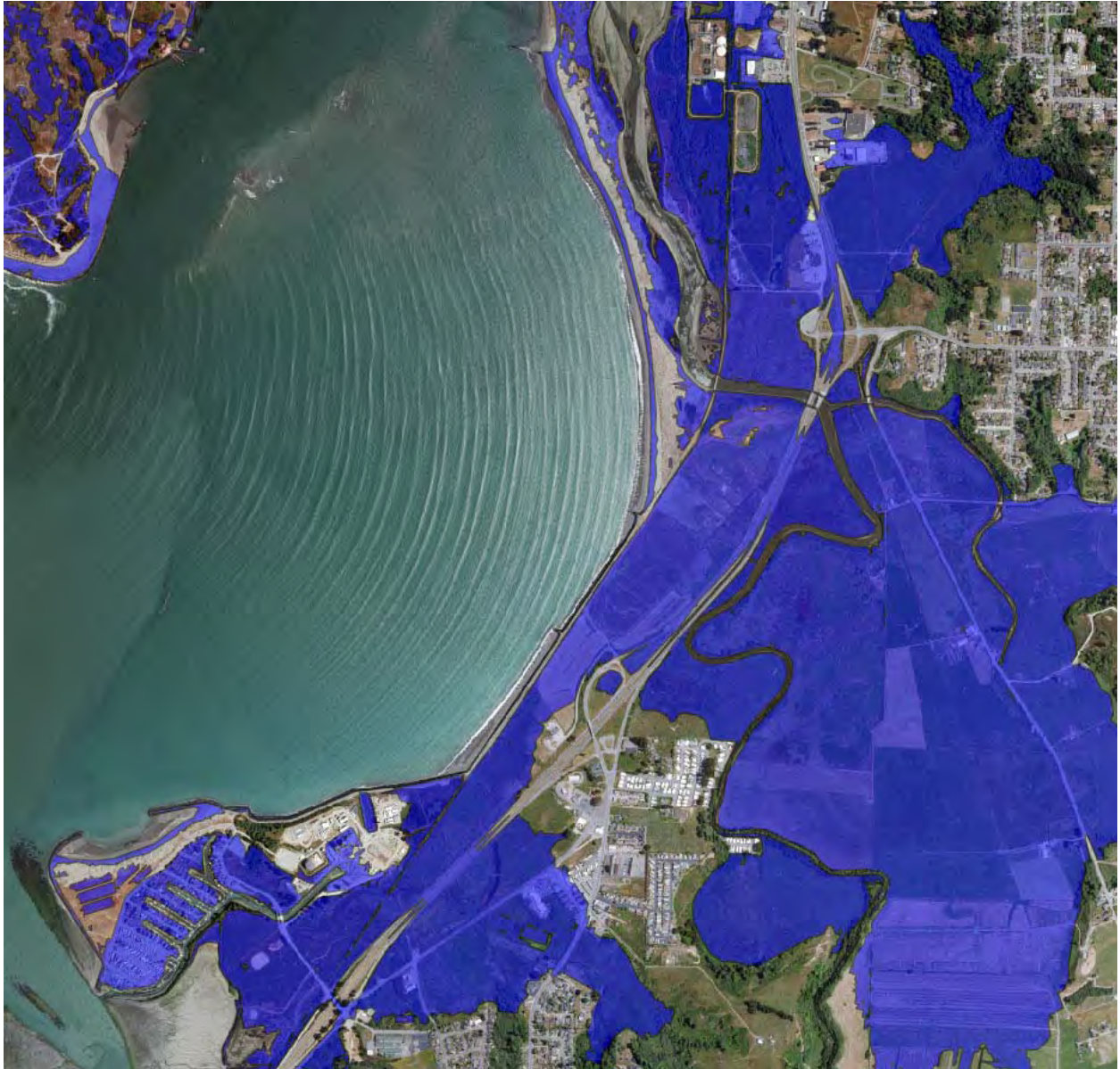
Figure 36. Middle segment by 2100, south of Eureka by 2100, could be tidally inundated by 4.9 ft. (1.5 M) of sea level rise. Both north and south bound lanes are almost entirely inundated.
