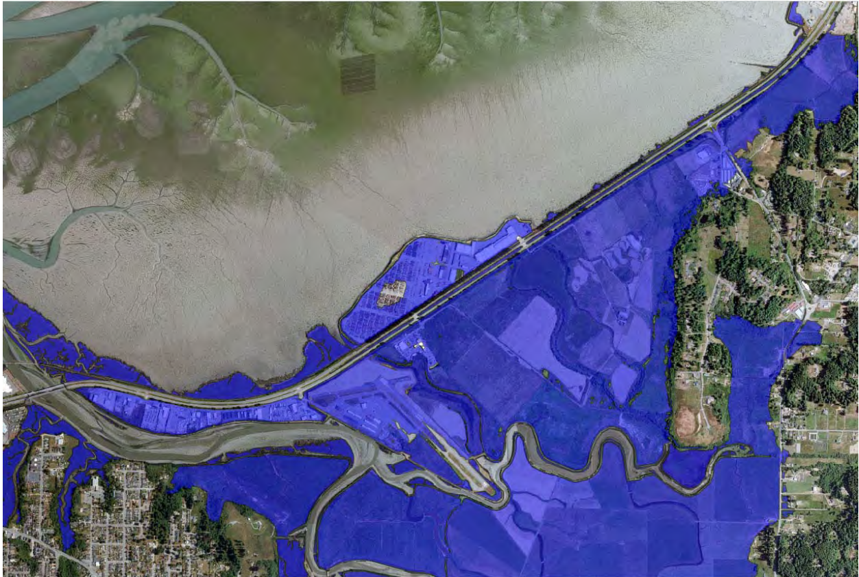
Figure 28. Lower reach of North segment with 0.9 ft. of sea level rise with a tidal elevation of 8.8 feet (MAMW). Should the protective shoreline structures be compromised, the land adjacent to the road prism could be inundated from the east of Highway 101. In the HBAP planning area, approximately 0.73 miles of the north bound lanes of the lower reach could become tidally inundated.
