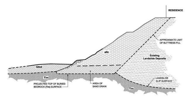
Without the continued existence of armoring at the site, the stabilization system will be susceptible to damage and destabilization from wave attack. The landslide movement during the heavy rainfall season of 1977-79 and the slope damage resulting from the severe El Niño storms of 1983 provide further evidence of the risk to the structures.
