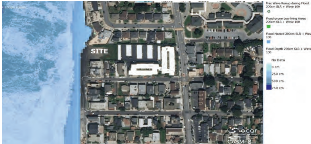
Figure 3. USGS CoSMoS wave overtopping analysis for 6.6 feet of SLR and the 100 year storm.
