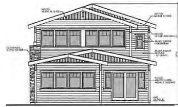
SOUTH ELEVATION SCALE: 1/4" = 1'-0"
