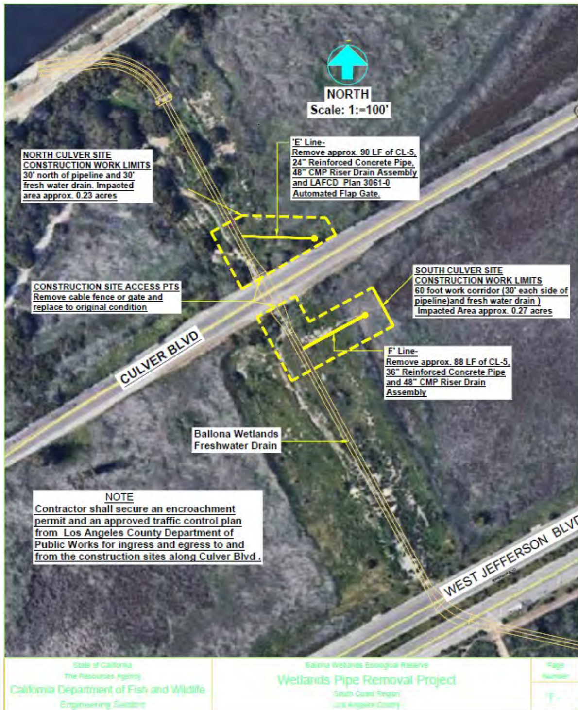
Figure 2. CDFW, Engineering Section, BWER Wetlands Pipe Removal Project exhibit (page number T -) that depicts the approximated areal extent of impact for removing the debris drain risers and pipes north and south of Culver Boulevard (that was used to calculate the mitigation acreage) and shows how the debris drain risers and pipes are connected with the freshwater marsh storm drain.
