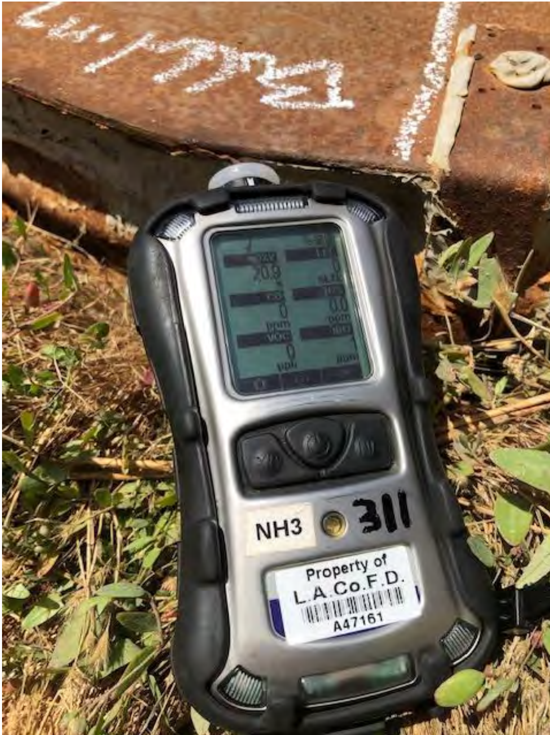
Figure 1: HazMat Meter Reading Directly in Front of South Drain Leak (all zero, except 20.9% oxygen and 1 ppm ammonia)
