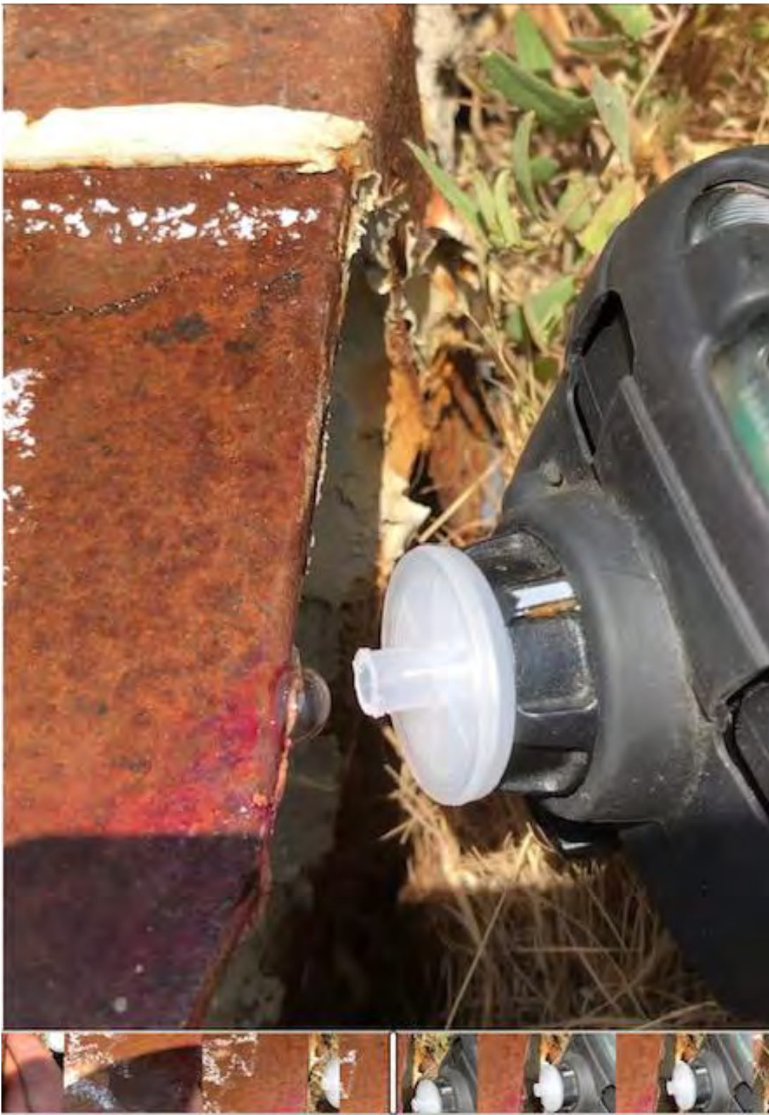
Figure 2: South Drain Reading Directly in Front of Air Leak (water poured over to expose leak)
