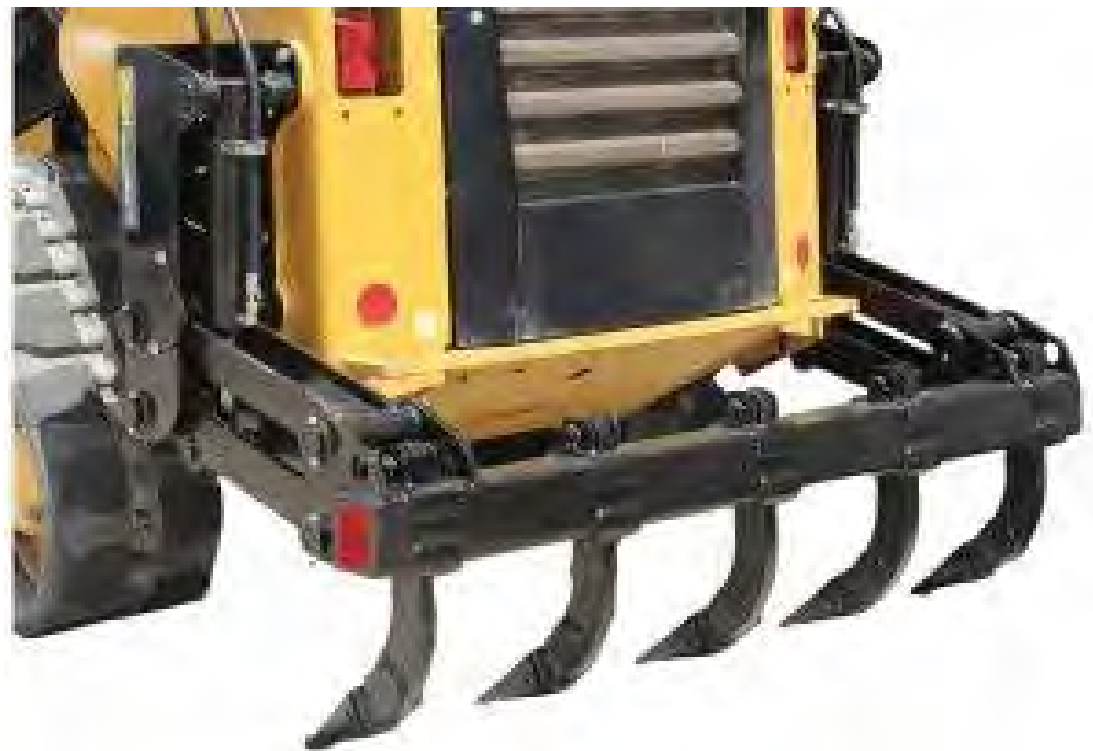
Figure 7-10. Tractor Ripper Attachment for Soil Decompaction by Ripping
