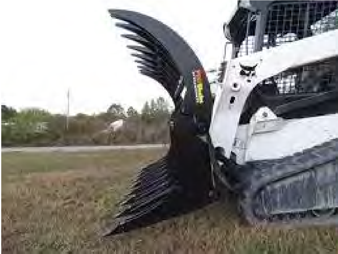
Figure 7-11. Bobcat with Root Rake Clam Grapple for Removal of Dense Iceplant Mats
