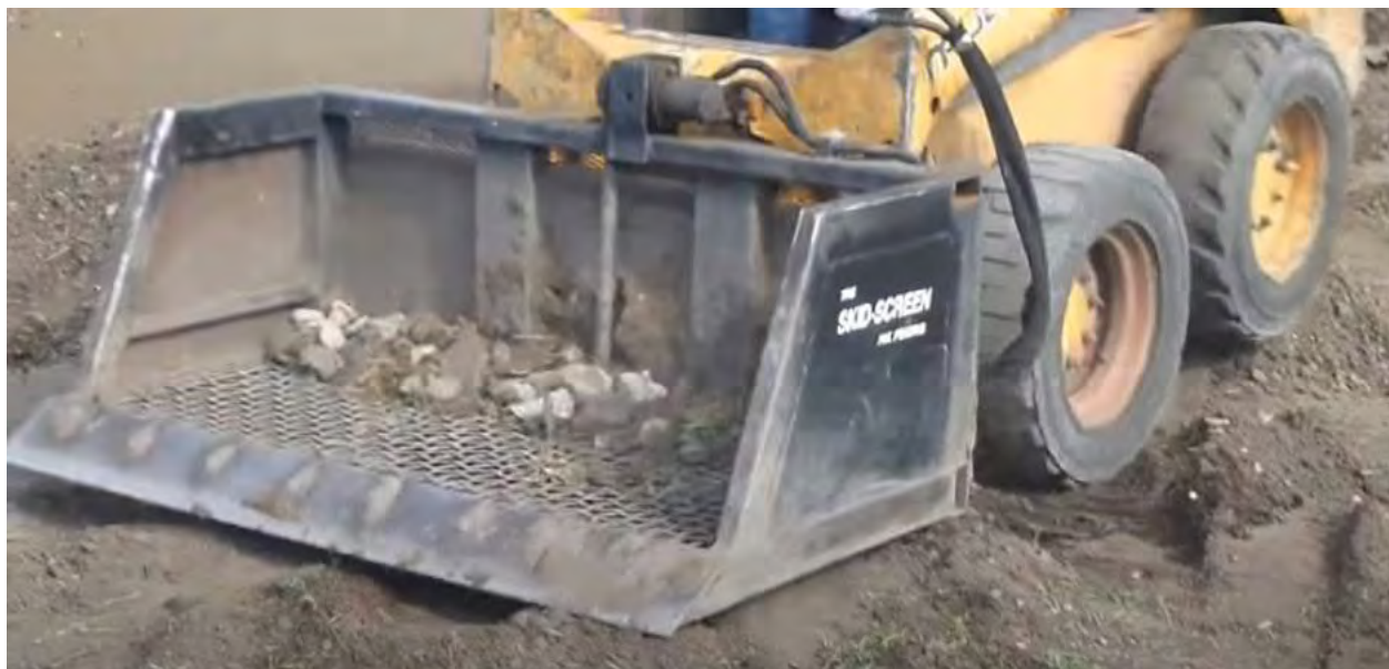
Figure 7-14. Bobcat with Vibratory Screen Bucket for Separation of Organic Iceplant Debris from Sand
