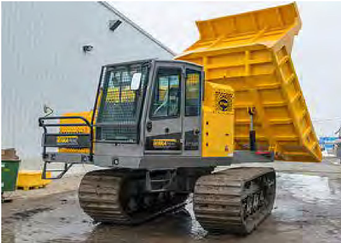
Figure 7-12. Light Ground Pressure Dump Truck for Removal of Iceplant Masses
