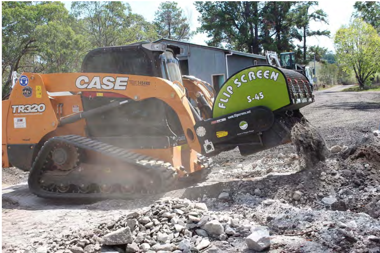
Figure 7-13. Bobcat with Flip Screen Bucket for Separation of Organic Iceplant Debris from Sand
