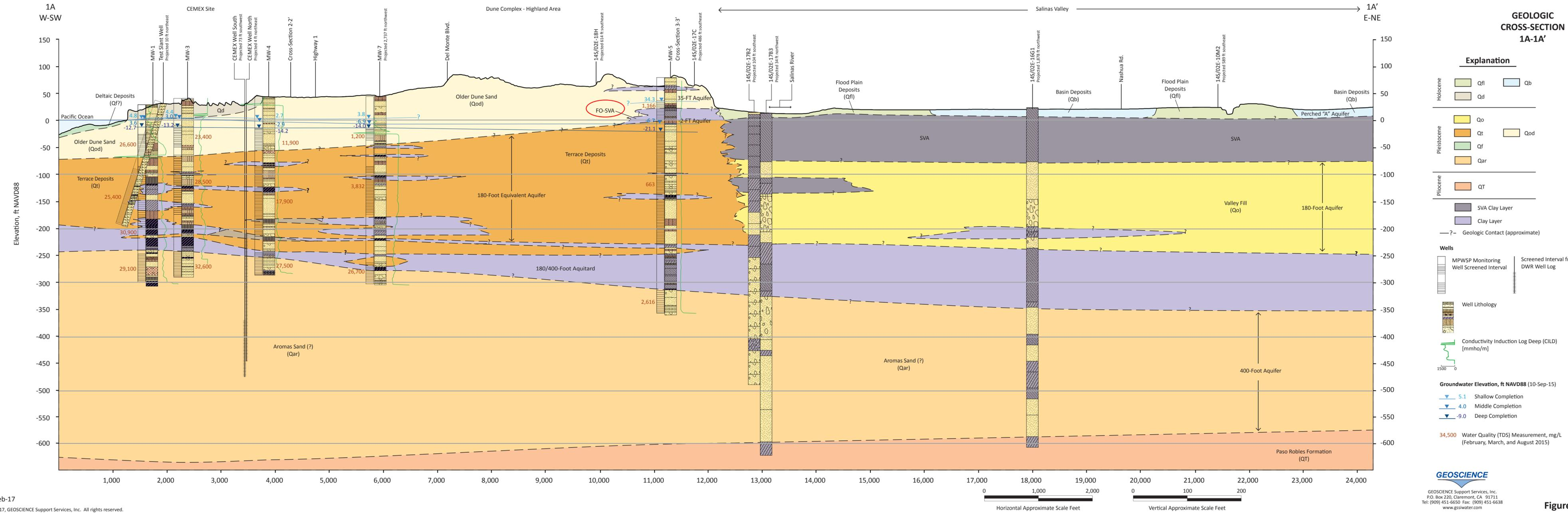
**GEOLOGIC CROSS-SECTION 1A-1A'**
