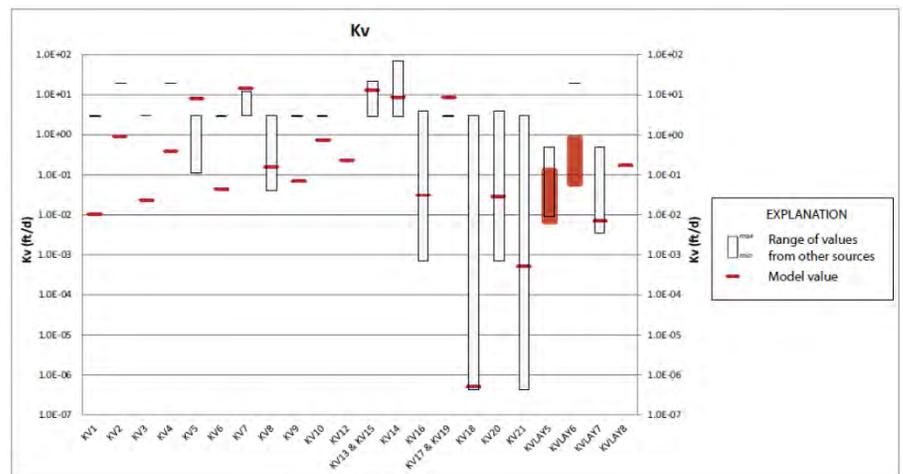
Vertical Hydraulic Conductivity (KV) Parameter Zones and Values, Model Layers 2 and 3, NMGWM<sup>2016</sup>, Excerpted from Figures 3.3b and 3.4b, *Final Environmental Impact Report/Environmental Impact Statement Appendix E2*, March 28, 2018. Red lines and text are added based on other figures in Appendix E2
