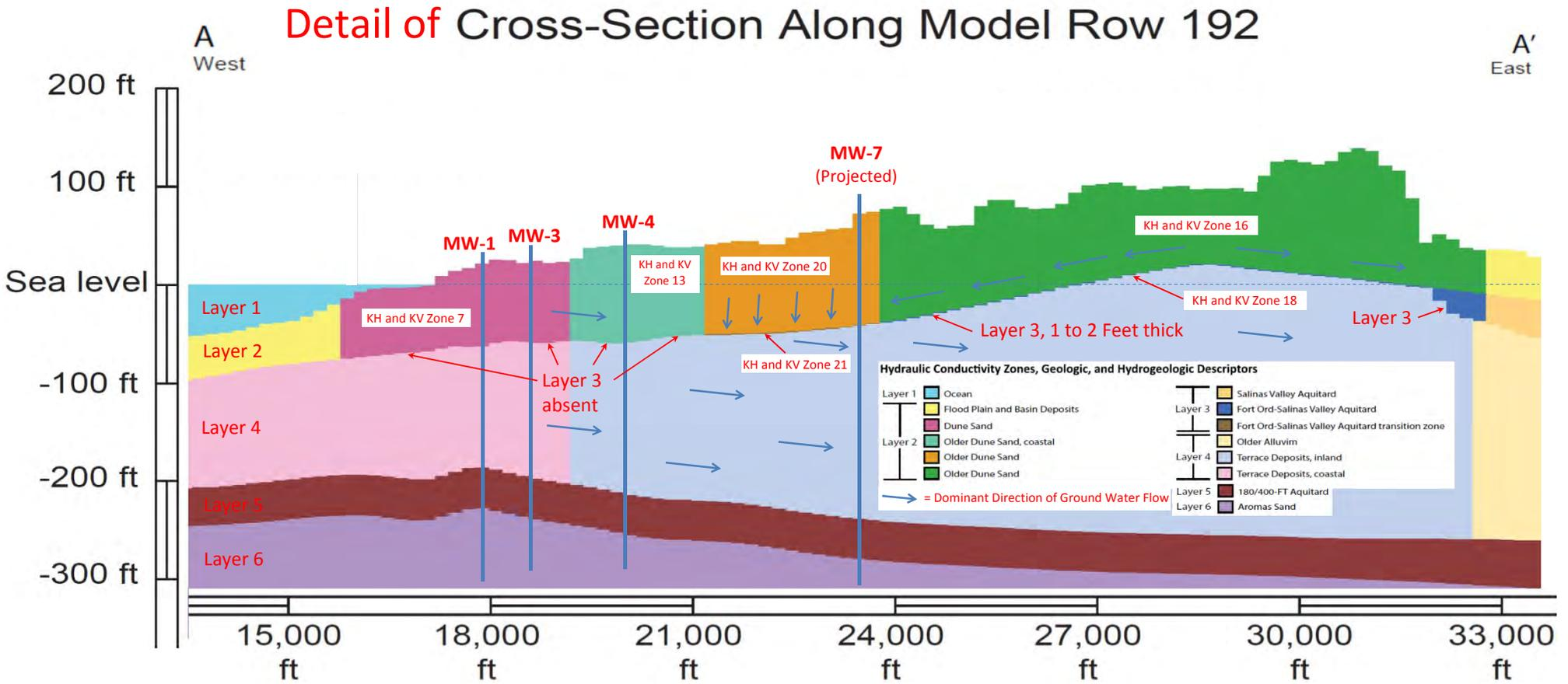
Hydraulic Conductivity Zones, Model Cross Section A-A', NMGWM<sup>2016</sup>, excerpted from Figure 3.2b, *Final Environmental Impact Report/Environmental Impact Statement Appendix E2*, March 28, 2018. Well and Layer notations are added based on other figures in Appendix E2
