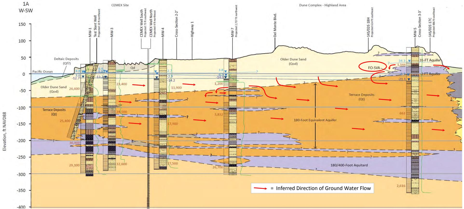
Excerpted from Figure 3, Geologic Cross Section 1A-1A', Monterey Peninsula Water Supply Project - Monitoring Well Completion Report and Cemex Model Update, Final EIR Appendix E3, annotations in red
