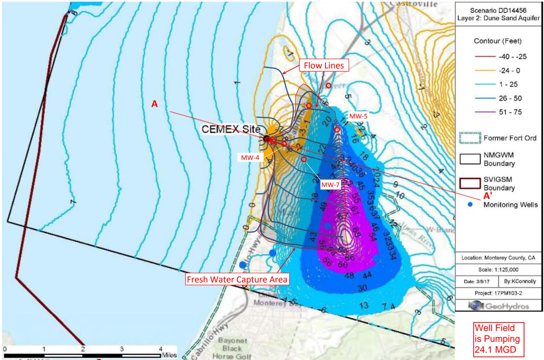
Figure 14. Simulated water table surface in the Dune Sand Aquifer (Layer 2) as portrayed by the calibrated version (top) and Scenario DD1-44/56 (bottom) showing mounding due to recharge in the Dune Sand Aquifer and equivalent fresh water heads assigned as constant values in the ocean resulting in a large eastward gradient across the model.
