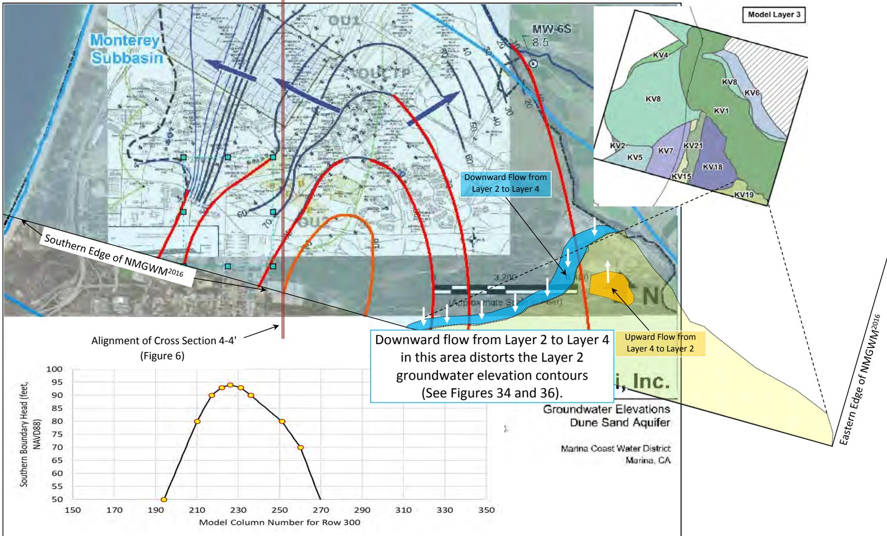
Figure 37. Vertical Groundwater Flow Through Layer 3, KV19
