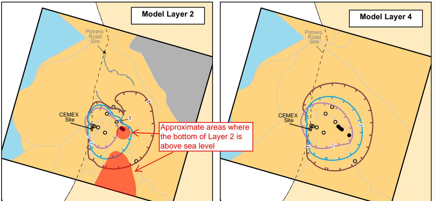
**Superposition Method Results for Model Layer 2 - Physical Inconsistencies - Example 2**
