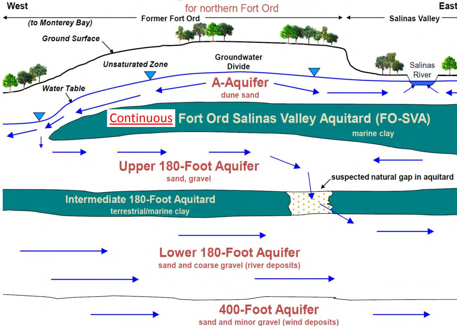
**Figure 1:** The Conceptual Site Model (Figure 1 at the left) describes groundwater conditions beneath former Fort Ord. Four aquifers are underlying former Fort Ord: A-Aquifer, Upper 180-Footer Aquifer, Lower 180-Footer Aquifer, and the 400-Footer Aquifer. Aquitards bound the A-, Upper 180-Footer Aquifer, Lower 180-Footer Aquifer, and 400-Footer Aquifers.
