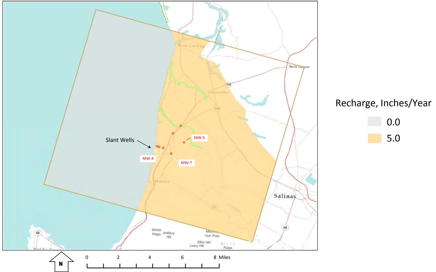
Figure 32. Area Where Recharge was Added to Layer 2 of NMGWM<sup>2016</sup>
