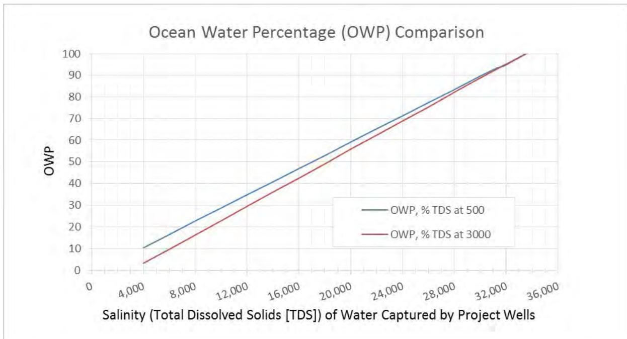
Given that the OWP during TSW testing rose above 90 percent long-term, and reflects the high end of the TDS range, the decrease in OWP calculated by assuming a fresh water standard of 3,000 mg/L instead of 500 mg/L is on the order of 1 to 2 percent.
