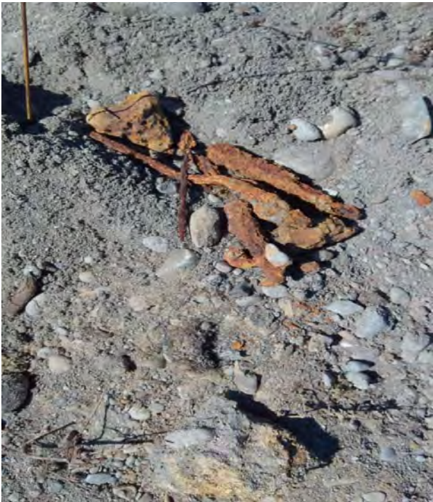
Photo 9: Iron debris contributing false "redox" colors at TPM2A.
