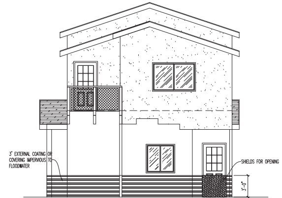
PROPOSED WEST ELEVATION - PASSIVE DRY FLOODPROOFING SYSTEM SCALE 1/4" = 1'-0"
