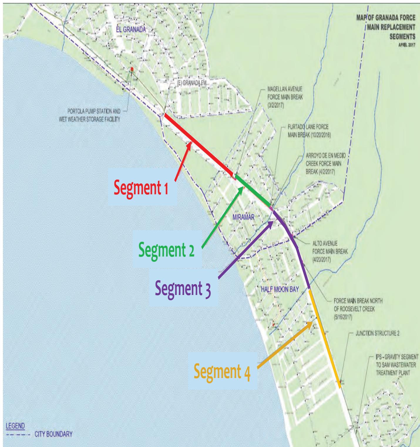
Figure 3. IPS Project Segments. Note the recent breaks in several force mains in Segments 1 to 3.
